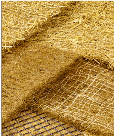
Figure A-9. Erosion control blankets made of natural fibers including straw and coir showing both natural and synthetic netting.
