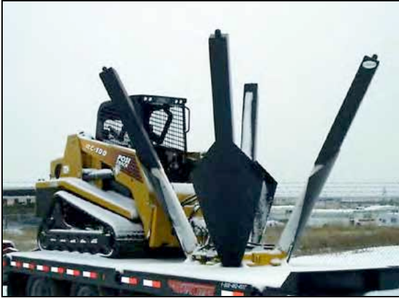
Figure A-19. Tree spade attachment for skid-steer.
